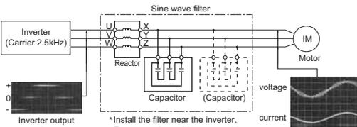
\* Install the filter near the inverter. For a capacitor cable, use a cable with size larger than indicated in the table below "recommended cable size".
