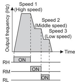
**Changing example** Operate at a high-speed (60 Hz).
