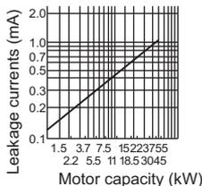
Example of leakage current per 1km during the commercial power supply operation when the CV cable is routed in metal conduit
