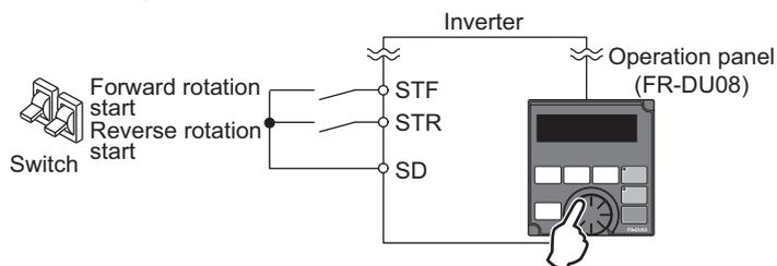
**Operation example** Operate at 30 Hz.
