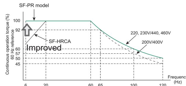
60 Hz torque reference indicates that the rated motor torque is 100% during 60 Hz operation.
