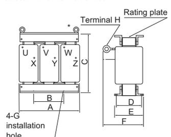
\* Remove the eye nut after installation of the product. This is a sample of the outer appearance, which differs depending on the model.
