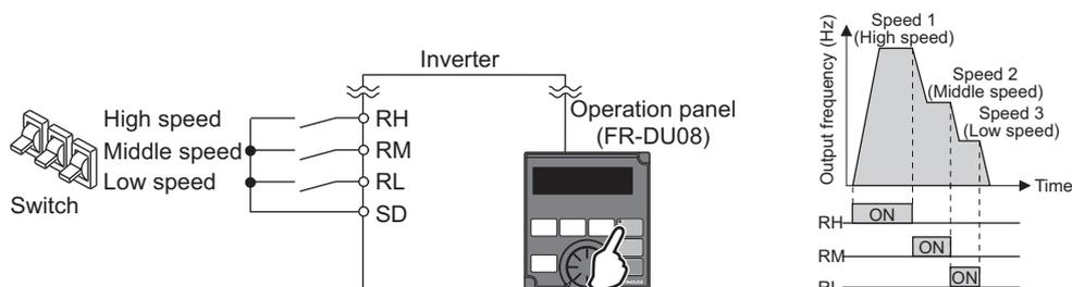
**Operation example** Operate at a low-speed (10 Hz).
