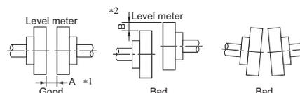
\*1 Set so that the A dimensions become the same dimension even when any position is measured by feeler gauge. (inequality in A width 3/100 mm or lower (2.5/100 mm or lower for MM-THE4))
