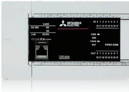
Maximum number of control points **512\*** points | Program capacity **64 k/128 k** steps | Pulse train **200 kpps** | Up to **4** axes
