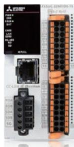
Maximum number of control points **512\*** points | Program capacity **64 k/128 k** steps | Pulse train **200 kpps** | Up to **4** axes
