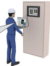
The personal computer and the GOT are connected with a USB cable or RS232 cable
